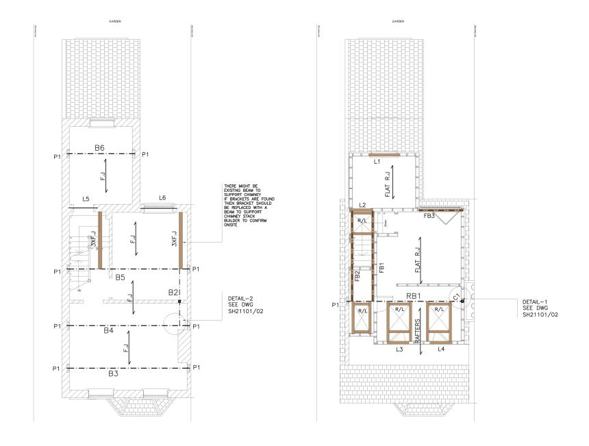
FIRST FLOOR PLAN SHOWING STRUCTURE OVER SCALE 1:100
